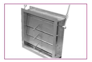
If the levers are set upward to ensure balance between the fins and the counterweight, the damper will be very sensitive and will open with minimal positive pressure exerted on the side opposite to the blade opening direction.
