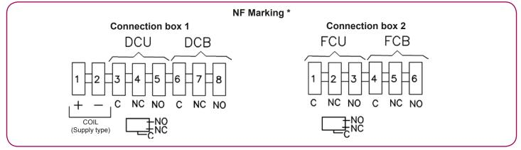
\* CE Marking does not require duplication of the start (DCU, DCB) and end of run limit switch (FCU, FCB).
