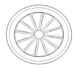
BLADE ANGLE POSITION OF 32° to 80° FOR WARM AIR ≥ 28°C (Adjustable by mechanic stop)
